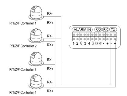
The RX/TX terminal of the reverse side of the SNS-110 uses the RS-442/485 interface and PAN/TILT/ZOOM/FOCUS controllers can be connected to the terminal.
